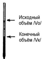
7. Measure the full volume of thiosulphate solution used for titration (both before and after adding the starch solution). In the case of obstructing impurities in the analyte water (suspended and colored substances, reducing agents, iron in concentrations above 1 mg/l), special sample treatment is required (see detailed description in the “Diluted oxygen” certificate). Then fill the oxygen flask with the sample, fix it, and titrate as described above.
