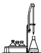
6. Collect 10 ml of thiosulphate solution into a burette (pipette) fixed in a holder from the kit and titrate the sample till light-yellow color. Then add 1 ml of starch solution (solution in the flask will become blue) with a pipette and keep titrating till the solution turns clear.
